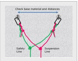
Anchor specification for Rope Access.
